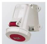
IP 67 wall-mounted receptacle with four exterior fastenings, entries - one on top and one blind (to cut out) at the bottom screwless spring terminal technology **TwinCONTACT**, connection terminals suitable for through wiring.
