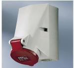
⚠ IP 44 wall-mounted receptacle, fastening from inside, entries - one on top and two blind (to cut out) at the bottom, lower part of housing can be rotated 180° screwless spring terminal technology **TwinCONTACT**, connecting terminals suitable for through wiring.
