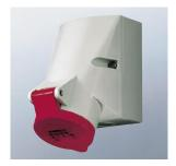
⚠ IP 44 wall-mounted receptacle, fastening from inside, entries - one on top and one blind (to cut out) at the bottom, lower part of housing can be rotated 180° screwless spring terminal technology **TwinCONTACT**, connecting terminals suitable for through wiring.
